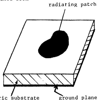
Fig. 1 Microstrip antenna configuration
