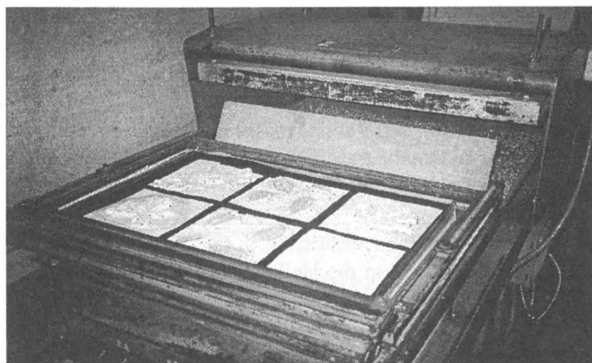
Figure 4. Vacuum press with molds of reconstructed Cretaceous leaves. Mylar sheets are sucked down on these molds and heated to conform to the molds. Then the leaves are hand-cut from the sheets by teams of volunteers.
