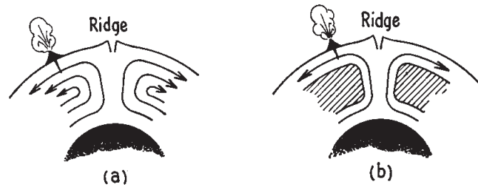
FIG. 4. Diagram to illustrate that in general if lava is generated at some other point of a convecting system than over a rising current, then only one volcano will be generated.
