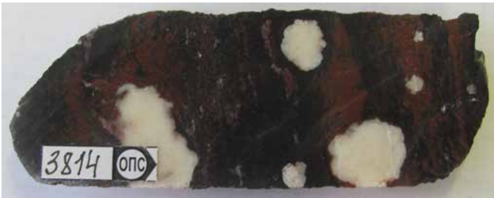
Fig. 6. Carbonate pseudomorphs after gypsum, core sample from the Onega Parametric Borehole. The sample is about 8 cm wide.
